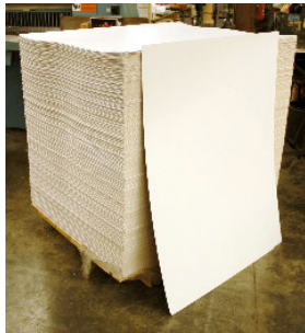
Image 4: a pallet of double white vat-lined chip courtesy of Burt Rigid Box
